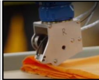
Figure 9: Robot end effector manipulating limp fabric (Source: ARM)
