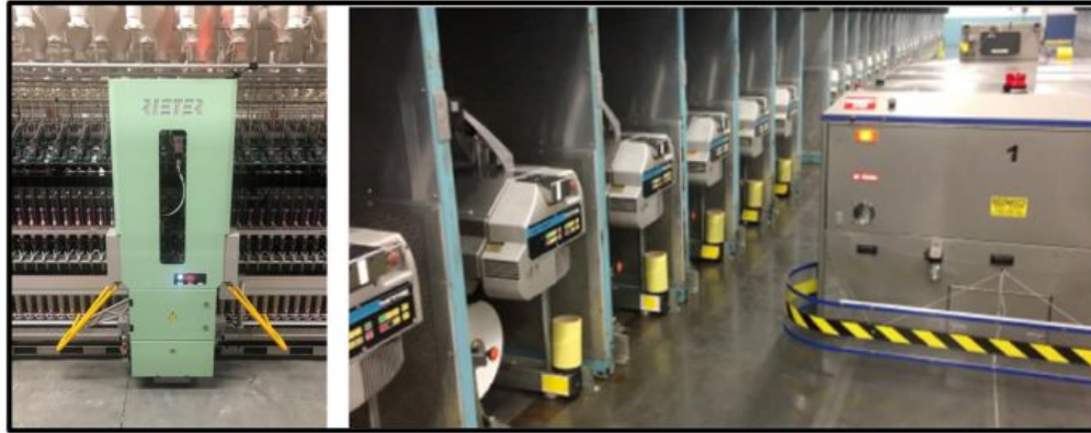
Figure 7: Automated ring spinning frame setup (Parkdale Mills) and yarn drawing & transport (UNIFI)
