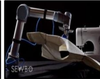
Figure 10: Robot manipulating stiffened fabric in a T-shirt manufacturing process (Source: Sewbo)
